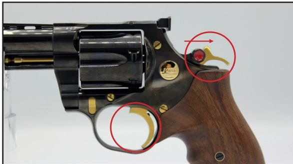
By pulling the hammer back until it latches, the cylinder rotates to the next chamber and the trigger moves backwards.
