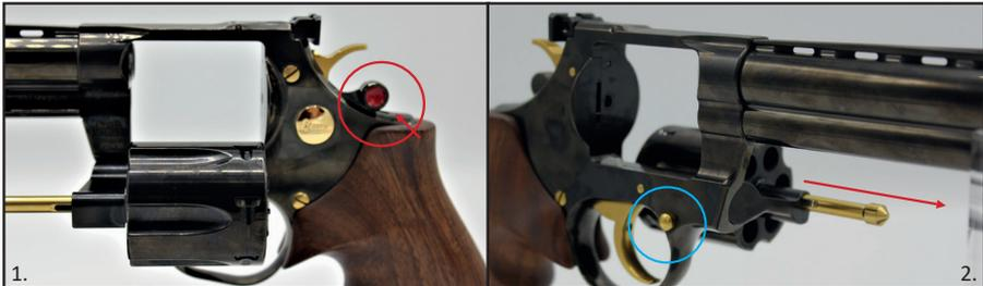
1. Press the thumbpiece forward towards the muzzle to release the extractor rod from the frame and swivel the cylinder to the left
