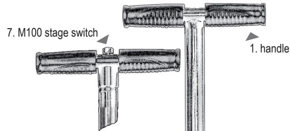
up to 150bar stage switch (7) on (counter clockwise)
